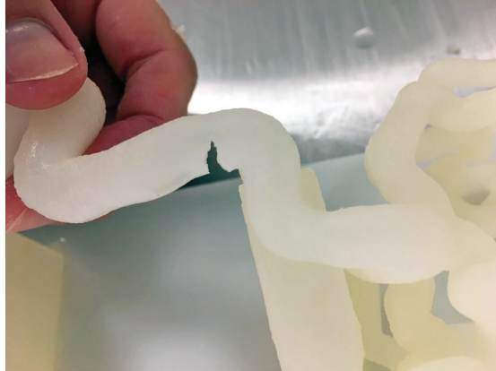
This tear in an early version of a 3D printed model guided new material development.
