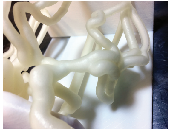
A 3D printed intracranial vasculature model printed with Agilus30.
