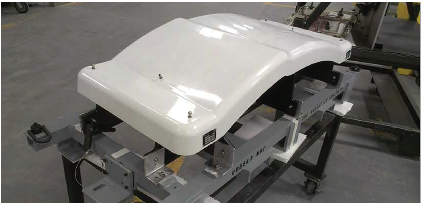
Figure 8. Original machining fixture made out of FRP composites.
