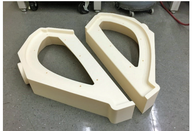
Figure 9. Mirrored halves of the FDM vacuum fixtures upon completion of printing.
